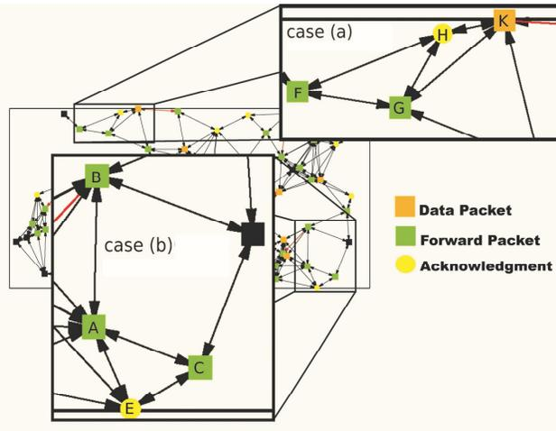
Fig. 1. Case (a): F, G and K transmit data to H. Case (b): A transmits data to B and C to E.
