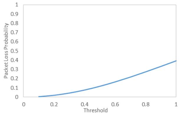
Fig. 2. Packet loss probability with scale = 1.
