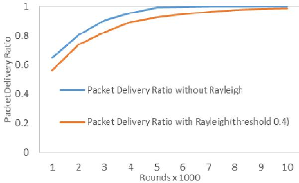
Fig. 3. Packets delivery ratio with Rayleigh fading. Threshold corresponds to signal level and packets are dropped in case that the signal level falls below 40% of the maximum signal strength during transmission.
